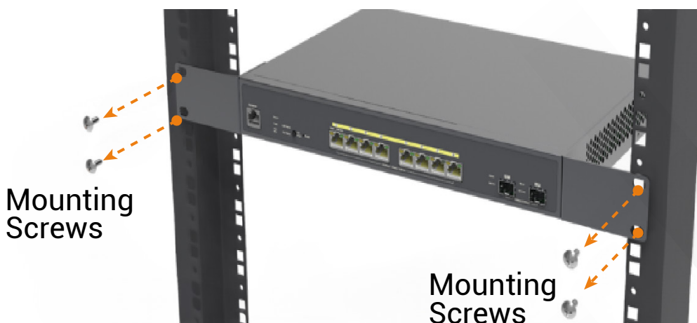
Installing the switch in a Rack
